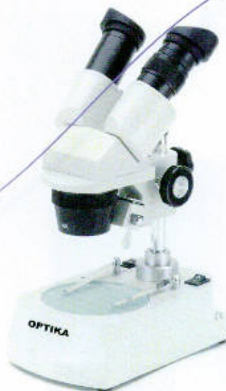
ST-30B-2L Stereomicroscope Head: Binocular, 45° inclined (rear) Eyepieces: WF10X/20mm Objective: 1x/3x Magnification: 10x/30x Illumination: Incident and transmitted 10W, tungsten bulbs
