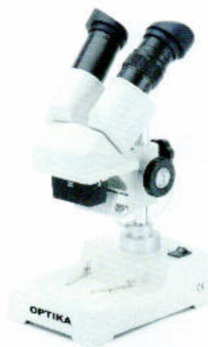
S-20-L Stereomicroscope Head: Binocular, 45° inclined (rear) Eyepieces: WF10X/20mm Objective: 2x Magnification: 20x Illumination: Incident 10W, tungsten bulb
